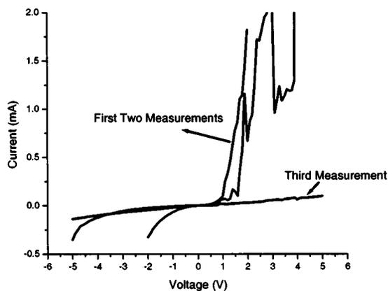
FIG. 3. Influence of an intentionally deposited aluminum oxide interface layer on the  $I$ - $V$  characteristics of Al contacts. The sample was a 15% N ASTEX-grown film. Measurements were performed in succession on the same pair of contact pads.
