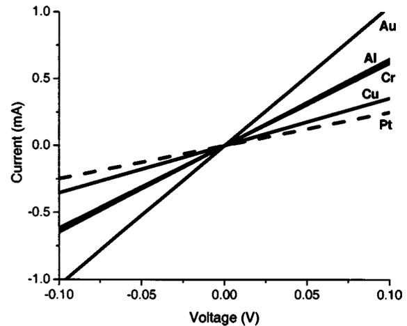
FIG. 1.  $I$ – $V$  characteristics for various metals on an as-grown 20% N UNCD film. The size and spacing of the contacts are identical in all cases.
