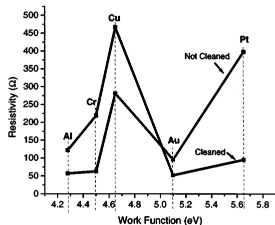
FIG. 2. Summary of  $I$ – $V$  characteristics for contacts deposited on both as-grown UNCD and acid cleaned UNCD. The same 20% N sample was used for all measurements shown here. The size and spacing of the contacts are identical in all cases. This shows the lack of monotonic dependence of  $R_{\text{contact}}$  on  $W$ . Results were similar for  $E_n$ .
