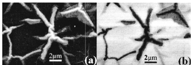
FIG. 2. Wire-island structures due to gallium spreading on 35 nm Au at 300°C. (a) Secondary electron and (b) backscattered electron SEM images at the boundary between zones 2 and 3. In (b) the image contrast has been inverted such that the dark regions correspond to the more dense Au-rich lamellae that are surrounded by and segregated from the lighter contrast Ga-rich lamellae.
