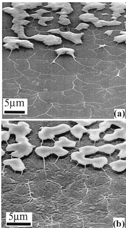
FIG. 3. Au-Ga structures in zones 2 and 3 (a) before and (b) after etching. The Ga was spread on 20 nm Au at 270°C. The SEM images are taken at 45° sample tilt. After etching the wires are released and are found suspended between the islands. Away from the islands, networks of nanowires are adhered to the substrate.
