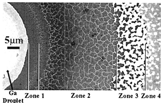
FIG. 1. Morphologies produced by the spreading of a gallium droplet on a 35 nm Au film at 300°C (SEM Image)—Ref. 7.
