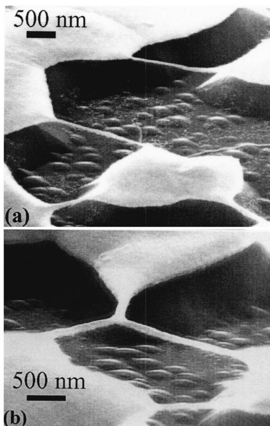
FIG. 4. Suspended Au–Ga nanowires in zone 3. (a) Four suspended wires. The diameter of the wire at the top of the image varies from 35 nm (left end) to 85 nm (right side). (b) A triple-wire structure with average width of 130 nm. The Ga was spread on 20 nm Au at 270°C.
