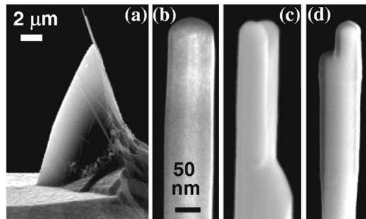
FIG. 2. Needles formed on cantilevers by the process of Fig. 1 (SEM images). (a) Closeup of the cantilever tip and attached needle from Fig. 1 and [(b)–(d)] closeups of single needles formed on three different tips. The scale bar in (b) also applies to (c) and (d).
