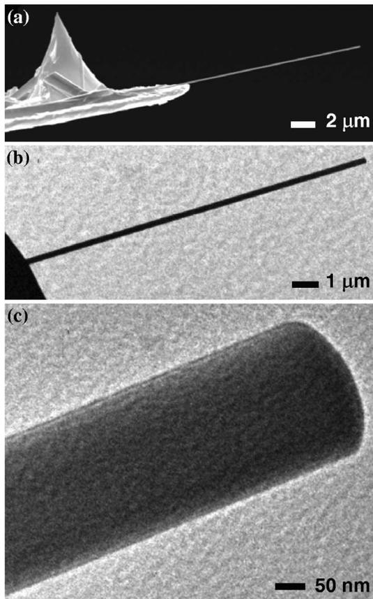
FIG. 4. Single needle that was selectively grown parallel to the surface of the cantilever. (a) SEM image of the  $\sim 250$ -nm-diameter needle showing that it protrudes  $14\ \mu\text{m}$  beyond the end of the cantilever. Closeup TEM images of (b) the entire length of the needle beyond the cantilever and (c) the end of the needle. These images show that the needle is of nearly constant diameter.
