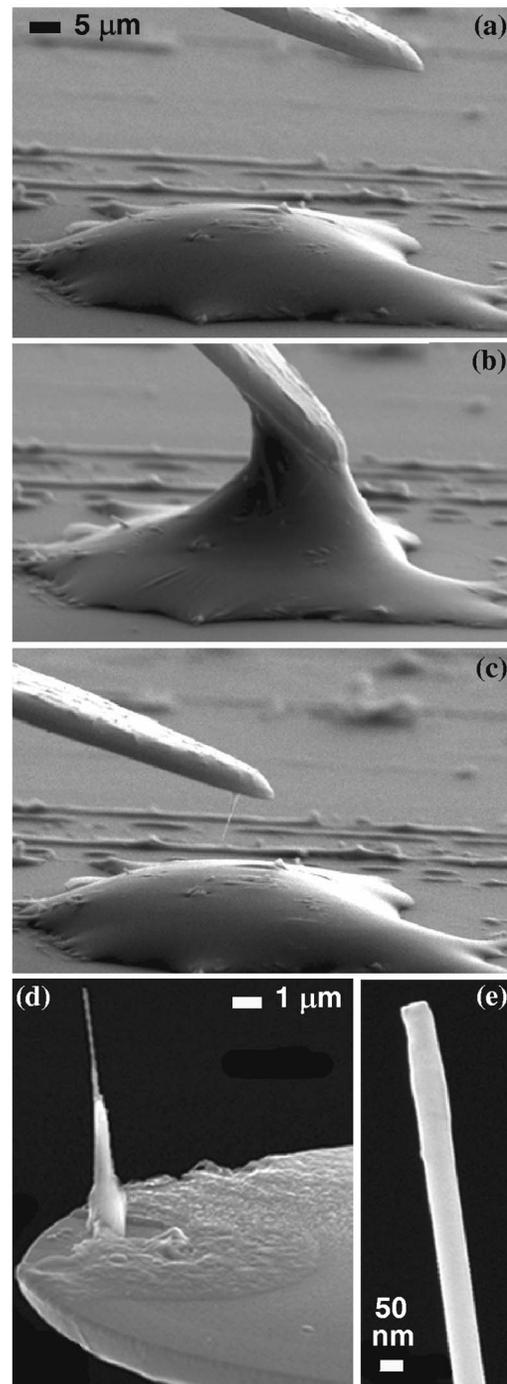
FIG. 5. Demonstration of the single-needle fabrication process on a tipless cantilever. [(a)–(c)] A sequence of SEM images that show the fabrication of the needle. (d) A closeup of the cantilever in (c) that shows that most of the Ag film has been removed around the base of the needle. (e) A further closeup of the needle formed on the cantilever. The end of the needle is  $55\ \text{nm}$  in diameter.
