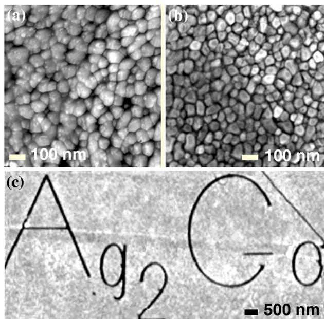
FIG. 7. Evaluations of the needle-tipped cantilevers for AFM applications. (a) AFM topography image of a thin sputtered Au film using a 120-nm-diameter needle-tipped cantilever. (b) SEM image of a similar looking area of the same film. Comparison of the two images, as described in the text, leads to an estimate that the tip resolution is 14 nm on this sample. (c) AFM image of pattern written with a needle-tipped cantilever by voltage lithography of a thin PMMA film.
