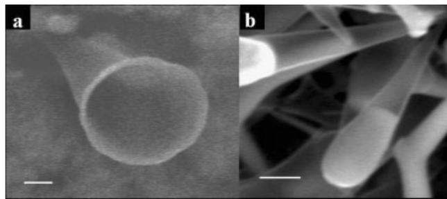
Fig. 2. Curved and tapered carbon tubular structures. Scanning electron microscopy (SEM) images of a) nozzles and b) cones synthesized upon exposing the prepared substrate to 18 %  $\text{CH}_4/\text{H}_2$  plasma. Scale bar: a) 500 nm, b) 2  $\mu\text{m}$ .
