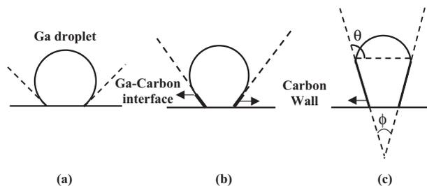
Fig. 1. Schematic of the growth mechanism. a) Initial gallium droplet, b) formation of carbon wall at the base of the gallium droplet. The wall forms tangential to the surface of the droplet. Addition of carbon occurs at the gallium carbon interface as shown. c) Geometric representation of the relation between the contact angle and the conical angle.
