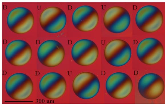
**Figure 6.** Optical image (using DIC) of buckled UP (U) and buckled DOWN (D) diaphragms ( $300\ \mu\text{m}$  diameter) for application as mechanical memory storage devices.
