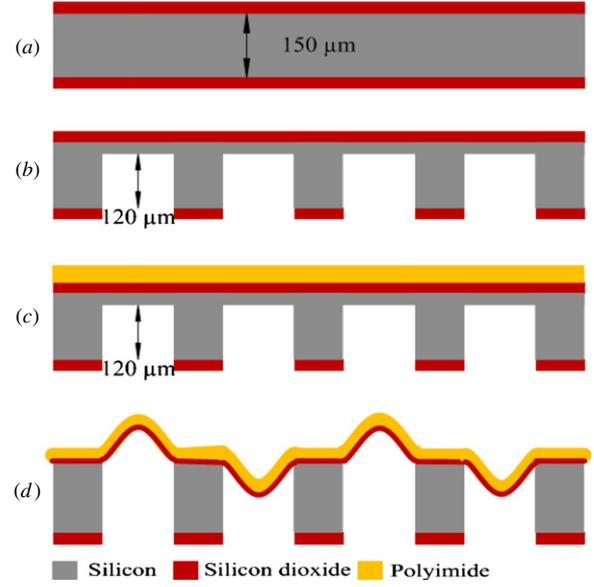
**Figure 1.** (a)  $300 \mu\text{m}$  thick DSP wafer wet-oxidized resulting in  $0.4 \mu\text{m}$  thick silicon dioxide. (b) Wafer patterned with  $300 \mu\text{m}$  diameter holes and DRIEed to etch  $120 \mu\text{m}$  silicon. (c) PI-2610 is spin-coated on the DRIEed wafer. (d) PI+oxide diaphragms are released by etching away (i.e. DRIE) the remaining silicon. Resulting diaphragms are either buckled UP or DOWN because of the compressive stresses in the oxide.
