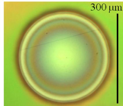
**Figure 5.** Optical image of concentric oxide circles resulting from the partially etched oxide during the second DRIE step. Shown here is the reverse side of the buckled oxide/PI diaphragm.
