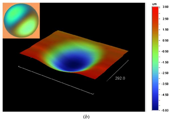
**Figure 2.** (a) Contact profile of the first state of the 300  $\mu\text{m}$  diameter buckled PI+oxide diaphragm (7.6  $\mu\text{m}$  buckling height). (b) 3D profile of the first state of a 300  $\mu\text{m}$  PI+oxide diaphragm (inset—optical image of the first state of the diaphragm using DIC).
