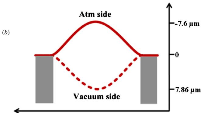
**Figure 4.** (a) Buckled UP (first state) diaphragm snapping DOWN (second state) at an actuating pressure of 41 kPa or 305 mmHg. Buckling height was measured using a contact profilometer for varying pressures (square markers—experimental data, solid line—theoretical data using equation (5)). (b) Buckled diaphragm in the first (UP) and second (DOWN) state.
