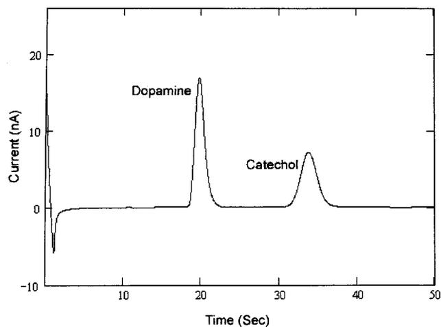
Figure 3. Electropherograms obtained for dopamine (2.2 mM) and catechol (2.3 mM) in pH 6 phosphate buffer for "optimum" microchip configuration. Conditions: CE voltage, 250 V; EC potential,  $+0.80$  V vs Pt wire.
