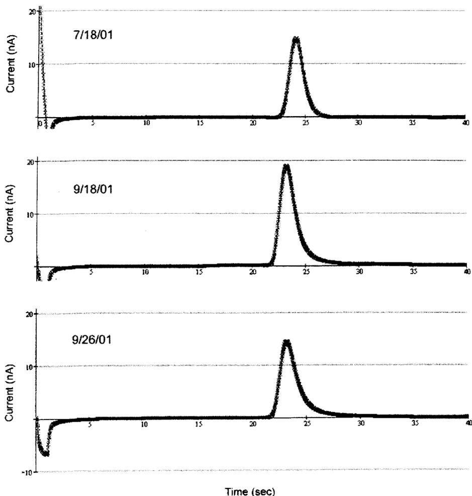
Figure 5. Electroperograms observed for dopamine (2.2 mM) with same microchip device on (A) 7/18/01, (B) 9/18/01, and (C) 9/26/01. Conditions as in Figure 3.
