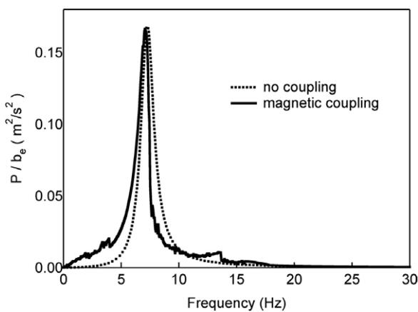
**Figure 7.** Simulated output of the piezoelectric cantilever for the case of no magnetic coupling (dashed line) and magnetic coupling (solid line).
