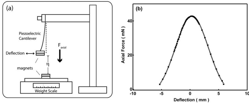
**Figure 6.** (a) Apparatus used to measure the axial magnetic force. (b) Axial force as a function of deflection distance for a 5 mm separation between the two magnets.
