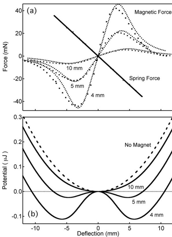
**Figure 5.** (a) The magnetic force  $F_B(\eta, z)$  for three separation distances ( $\eta = 4, 5$  and  $10$  mm). The lines show fits to equation (2). Also shown (as a straight line) is the spring force of the cantilever. (b) The cantilever spring potential (dashed line) and the potential due to the combination of the restoring force and the magnetic force for the three separation distances.
