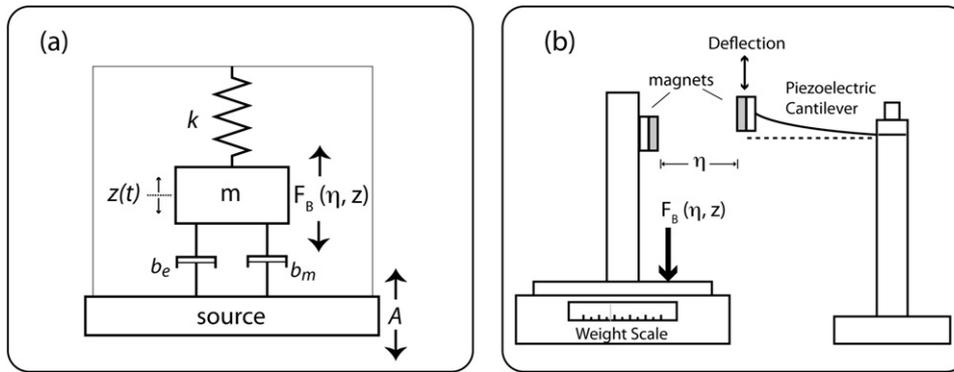
**Figure 4.** (a) Modified one-dimensional spring force model.  $A$  is the source acceleration,  $k$  is the spring constant,  $m$  is the proof mass,  $z(t)$  is the cantilever deflection and  $F_B(\eta, z)$  is the magnetic force. (b) Apparatus used to measure the magnetic force  $F_B(\eta, z)$ .
