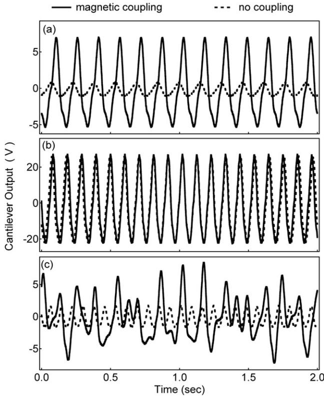
**Figure 3.** Non-rectified time domain voltage output of the cantilever (a) below resonance, using 6.5 Hz vibration frequency (b) at resonance, using 10 Hz vibration frequency and (c) above resonance, using 13 Hz vibration frequency.
