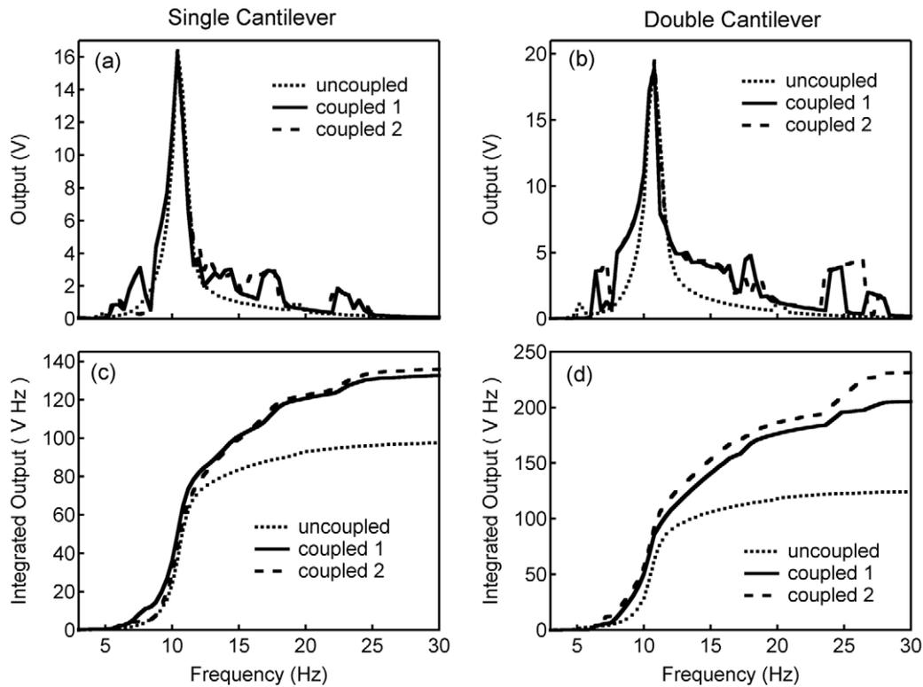
**Figure 2.** Voltage output of the piezoelectric cantilever as a function of shaker table frequency for (a) single cantilever (b) double cantilever. Integrated voltage output as a function of frequency for (c) single cantilever and (d) double cantilever.
