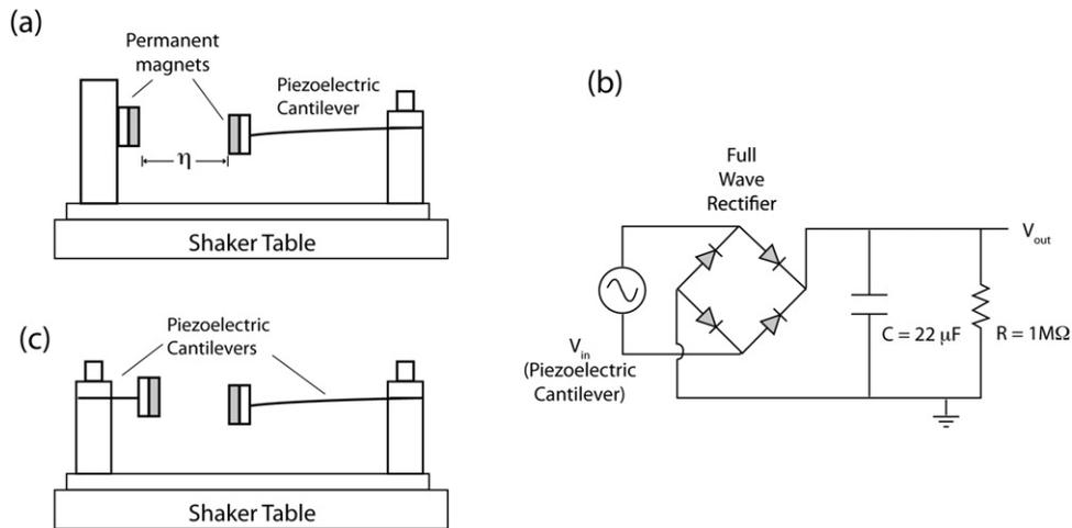
**Figure 1.** (a) Set-up with fixed opposing magnet. (b) Measurement circuit. (c) Set-up with opposing magnetic attached to a second cantilever.
