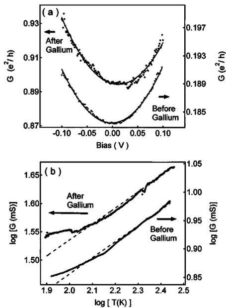
FIG. 3. (a) Differential conductance as a function of bias of a MWNT measured before and after the formation of the gallium contacts at 77 K. (b) Zero bias differential conductance as a function of temperature of a MWNT measured before and after the formation of the gallium contacts. The results are plotted on a log-log scale to bring out the power law dependence of the conductance on temperature.
