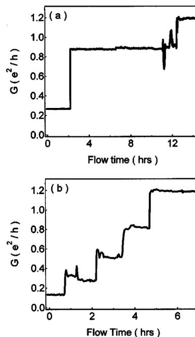
FIG. 2. Zero bias differential conductance of multiwall carbon nanotube measured at  $T=320$  K as a function of gallium flow time. A jump in conductance is observed each time the gallium makes contact with one end of a nanotube. (a) A single MWNT lies across a pair of gold leads, (b) two MWNTs lie across a pair of gold leads.
