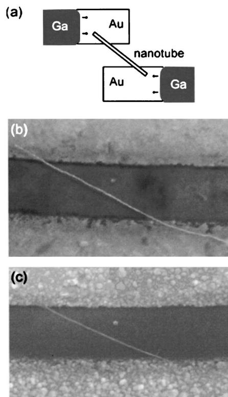
FIG. 1. (a) Schematic drawing showing our device layout. The conductance across the nanotube is monitored as gallium flows along the nanotube leads. Scanning electron microscope images of a nanotube device (b) before and (c) after gallium flows across the gold leads. The contact separation is approximately 1 μm. The contact resulting following gallium flow is an alloy of gold and gallium throughout its entire thickness.
