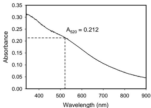
Fig. 3. UV-Vis absorbance spectrum of a C8/MUA MPC film deposited on glass after subtraction of a bare glass spectrum. The absorbance decreases with increasing wavelength and there is a small, broad peak near 550 nm, consistent with the assembly of tiny, aggregated clusters in the film. Absorbance was measured at 520 nm for the MPC concentration and edge-to-edge spacing analysis.
