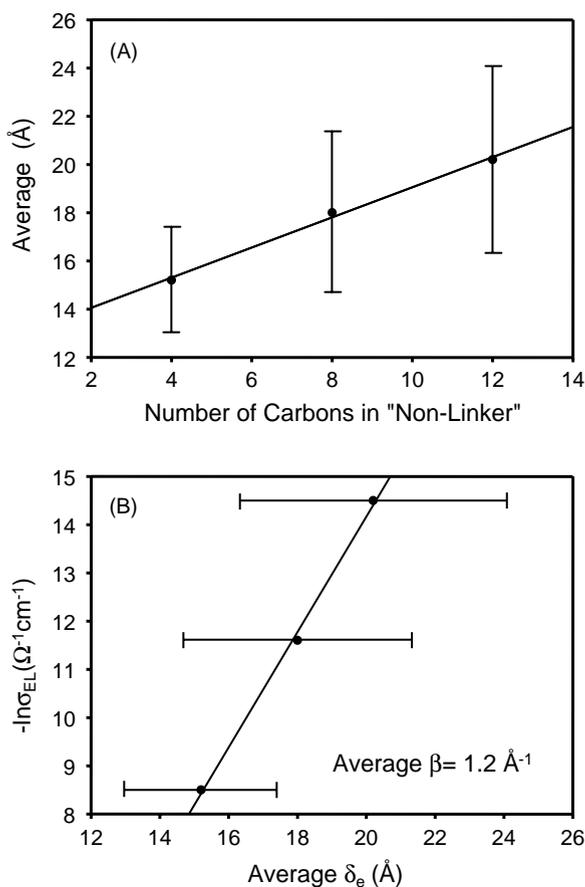
Fig. 4. (A) Plot of average edge-to-edge distance ( $\delta_e$ ) vs. the number of carbons in the non-linker chainlength and (B)  $-\ln(\sigma_{EL})$  vs.  $\delta_e$  for the various MPC films studied (C4/MUA, C8/MUA, and C12/MUA). The data are displayed in Tables 1 and 2.  $\delta_e$  increases linearly with increasing chainlength and  $\sigma_{EL}$  increases exponentially with decreasing chainlength (or decreasing  $\delta_e$ ) as expected for a electron tunneling process.
