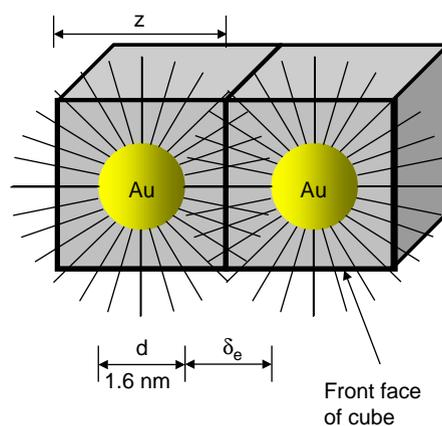
$$\begin{aligned} \delta_e &= z - d \\ &= (1/C_{\text{MPC}})^{1/3} - 1.6 \times 10^{-7} \text{ cm} \end{aligned}$$
