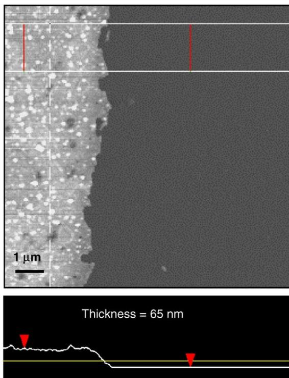
Fig. 2. An AFM image (top) showing the edge of a patterned C8/MUA MPC film on an Au substrate and the corresponding cross-sectional line scan (bottom) used to obtain the film thickness. This film was 65 nm thick.
