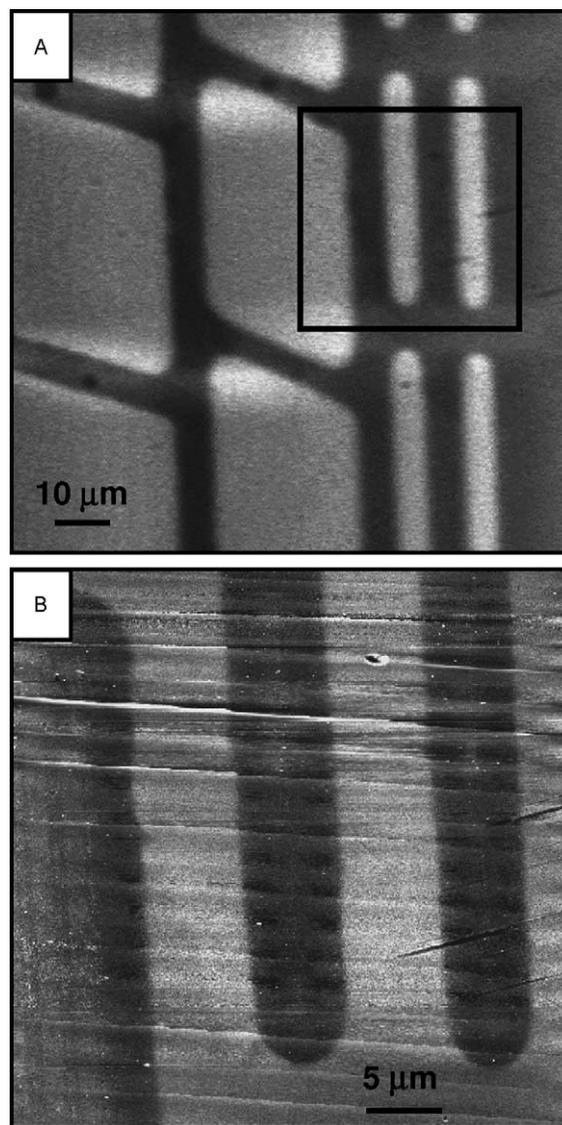
Fig. 1. (A) Optical and (B) AFM image of a C6/MUA MPC film microcontact printed on an Au substrate. The film was deposited using two dip cycles and the procedure outlined in Scheme 1. The square in Frame A corresponds to the approximate area imaged with AFM in Frame B. Opposite contrast is observed for the two images due to the different imaging mechanisms. Au/C16S regions appear bright in the optical image, but dark in the AFM image, and vice versa for the Au/MPC regions.
