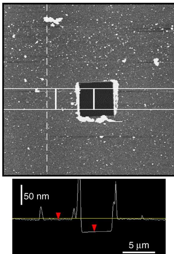
Fig. 7. A tapping-mode AFM image showing a  $5\ \mu\text{m} \times 5\ \mu\text{m}$  square pattern that was fabricated on a C12/MUA MPC film on an Au substrate with a Pt/Ir STM tip. The pattern was prepared by scanning the area for 15 min at a bias of 0.5 V and tunneling current of 1.0 nA. The cross-sectional line scan shows that the thickness of the film was approximately 31 nm.
