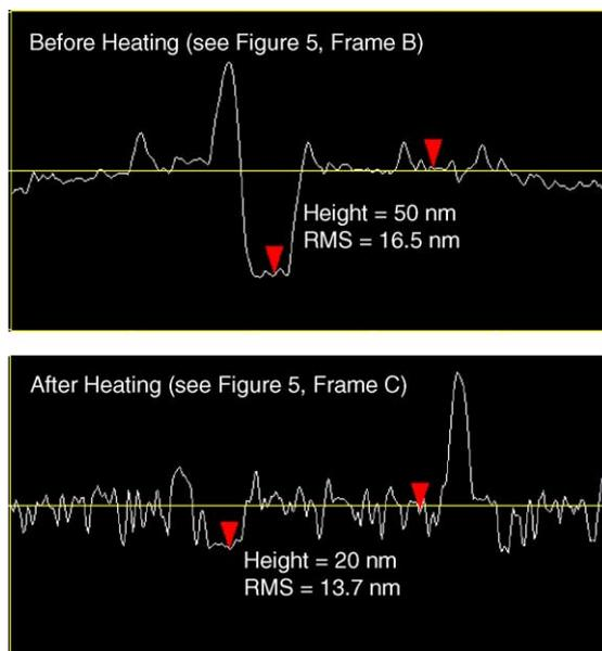
Fig. 6. Cross-sectional line scans of the  $1\ \mu\text{m} \times 1\ \mu\text{m}$  pattern from Fig. 5 (Frames B and C) before and after heating (top and bottom frames, respectively). The film becomes smoother and the thickness decreases from 50 to 20 nm (60%) upon heating.
