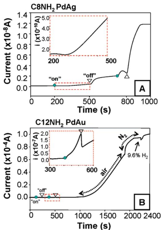
**Figure 5.** CA plots of films of (A) C8NH<sub>2</sub> PdAg and (B) C12NH<sub>2</sub> PdAu measured at  $-0.3$  V during repeated exposure to 100% H<sub>2</sub> (●) and air (△) during film conditioning to reach stable currents. (Insets) Expanded plots of the regions indicated by the dashed rectangles.
