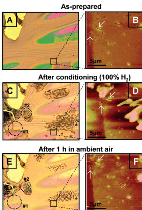
**Figure 8.** Optical (A, C, E) and AFM (B, D, F) images of a film of C8NH<sub>2</sub> Pd MPCs before (A, B) and after (C, D) conditioning by exposure to 100% H<sub>2</sub> for 500 s and air for 200 s. (E, F) shows the same film after an additional 1 h exposure to air. Circles labeled #1 represent areas where the film healed, and circles labeled #2 represent areas where the films changed irreversibly after exposure to 1 h in air.
