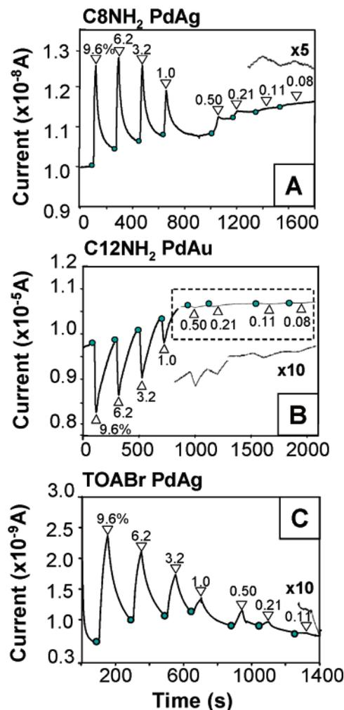
**Figure 6.** CA plots of films of (A) C8NH<sub>2</sub> PdAg MPCs, (B) C12NH<sub>2</sub> PdAu MPCs, and (C) TOABr PdAg nanoparticles exposed to H<sub>2</sub> concentrations from 9.6 to 0.08% as indicated in N<sub>2</sub> carrier gas. The films were initially exposed to 100% N<sub>2</sub>, and the circles represent the point of exposure to the H<sub>2</sub> concentration indicated and open triangles represent the point of exposure back to 100% N<sub>2</sub>.
