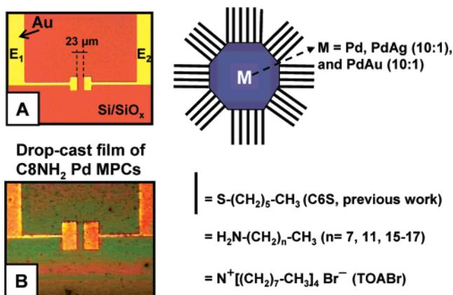
**Figure 1.** Optical microscope images of the electrode device (A) before and (B) after drop-cast deposition of a film of C<sub>8</sub>NH<sub>2</sub> Pd MPCs between the 23 μm electrode gap. The scheme of the nanoparticle shows the different metal compositions and different ligand stabilizers used in our previous work (C<sub>6</sub>S Pd MPCs) and this report (alkylamine- and TOABr-coated Pd and Pd alloy nanoparticles).
