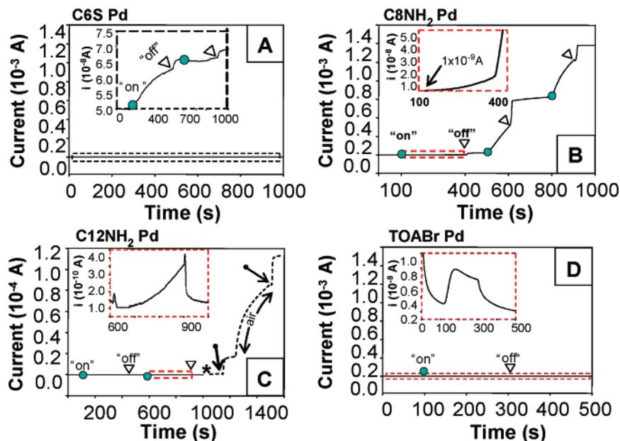
**Figure 3.** CA plots of films of (A) C6S Pd MPCs, (B) C8NH<sub>2</sub> Pd MPCs, (C) C12NH<sub>2</sub> Pd MPCs, and (D) TOABr Pd nanoparticles measured at  $-0.3$  V during repeated exposure to 100% H<sub>2</sub> (●) and air (△) during film conditioning to reach stable currents. (Insets) Expanded plots of the regions indicated by the dashed rectangles. The arrows after the \* in (C) represent exposure to 9.6% H<sub>2</sub>.
