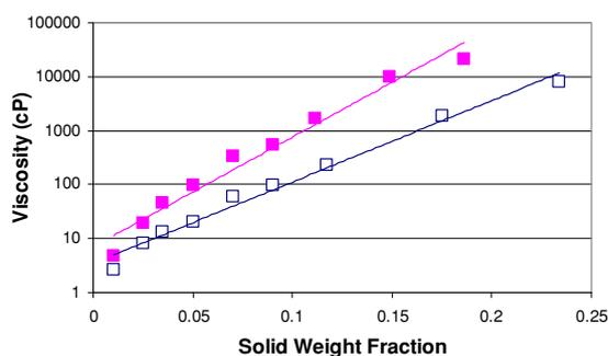
**Figure 2.** Viscosity of PMMA solution as a function of concentration. The upper and lower measured data and regression curves ( $\eta = 3.476 e^{34.721SWF}$  with  $R^2 = 0.9847$  and  $\eta = 7.0256 e^{46.828SWF}$  with  $R^2 = 0.9704$ ) are for the 950 k MW and 495k MW PMMA solutions, respectively.
