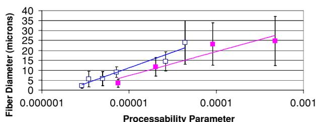
**Figure 11.** Fiber diameter as a function of the processability parameter. The data and fit are for the 950k g mol<sup>-1</sup> solution (upper curve) and the 495k g mol<sup>-1</sup> (lower curve) solutions.
