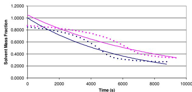
**Figure 3.** Solvent mass fraction for PMMA-chlorobenzene solutions as a function of time and molecular weight. The lower dotted and upper dotted lines represent the actual data recorded by the TGA for the  $495 \text{ k g mol}^{-1}$  polymer and  $950 \text{ k g mol}^{-1}$  polymer, respectively. Exponential regression analysis, indicated by the lower and upper solid lines, respectively, was performed on the TGA data in order to calculate the processability parameter.
