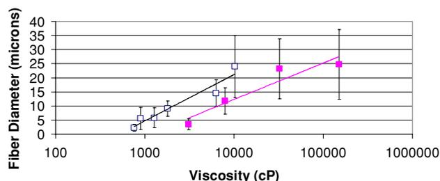
**Figure 10.** Fiber diameter as a function of viscosity. The data and fit are for the 950k g mol<sup>-1</sup> solution (upper curve) and the 495k g mol<sup>-1</sup> (lower curve) solutions.
