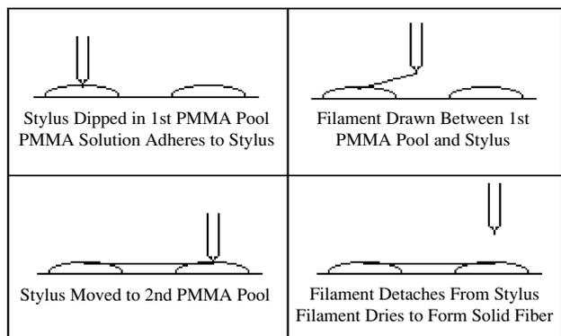
**Figure 1.** Schematic of the method of drawing micro- and nanofibers between two solvated PMMA pools.
