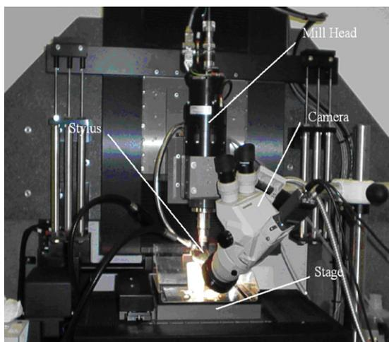
**Figure 5.** Dover instruments micromilling machine—the stage which contains the substrate material translates in the horizontal plane whereas the stylus, which is attached to the mill head, translates vertically.
