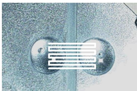
**Figure 4.** Solution deposited on silicon substrate immediately before trial run. The line indicates the serpentine path taken by the stylus.
