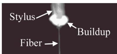
**Figure 8.** PMMA build-up on tungsten stylus accumulated during a single characterization trial.
