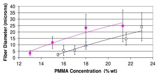
**Figure 7.** Fiber diameter versus concentration. The hollow and solid data points represent the average measured diameters of the drawn fibers for the  $495\text{k g mol}^{-1}$  data and the  $950\text{k g mol}^{-1}$  data, respectively. The error bars represent the standard deviation of each data point.
