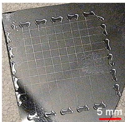
**Figure 9.** Weave pattern generated by the direct-write technique with 23% 495k g mol<sup>-1</sup> PMMA solution.
