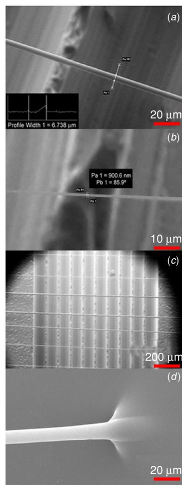
**Figure 6.** SEM images of polymer fibers drawn over a 1.8 mm trench. (a) Suspended fiber drawn from 15% solution of  $950\text{k g mol}^{-1}$  PMMA. (b) Suspended fiber drawn from 13% solution of  $950\text{k g mol}^{-1}$  PMMA. (c) Several parallel fibers drawn from 15.5% solution of  $495\text{k g mol}^{-1}$  PMMA. (d) Tapered end of PMMA fiber.
